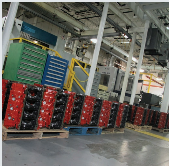
This must have been LSX day at the race lab, as pallets of them sat awaiting machining. In the race lab, for COPO use, these blocks are decked, their cam- and main-bores are machined, and their cylinder bores are machined and honed.
