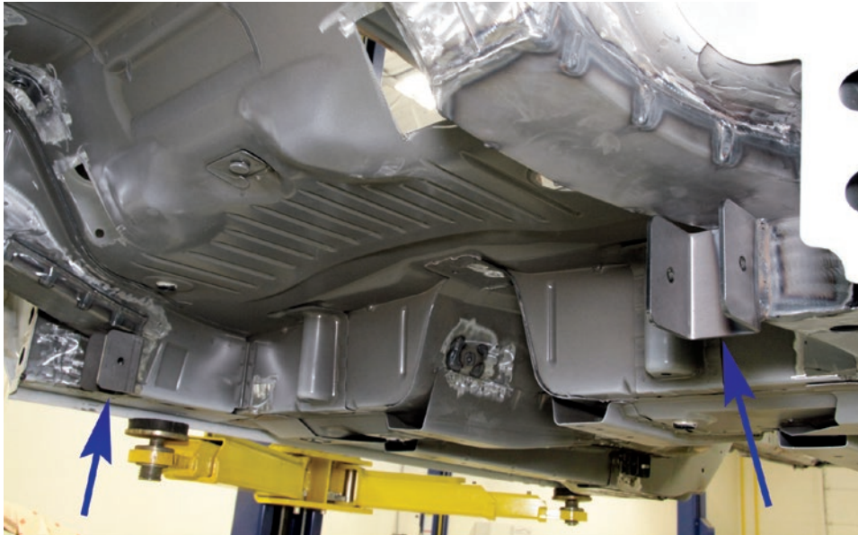
An overall look at the finished revisions to the subframe structure and the (arrows) attached lower control-arm chassis brackets.
