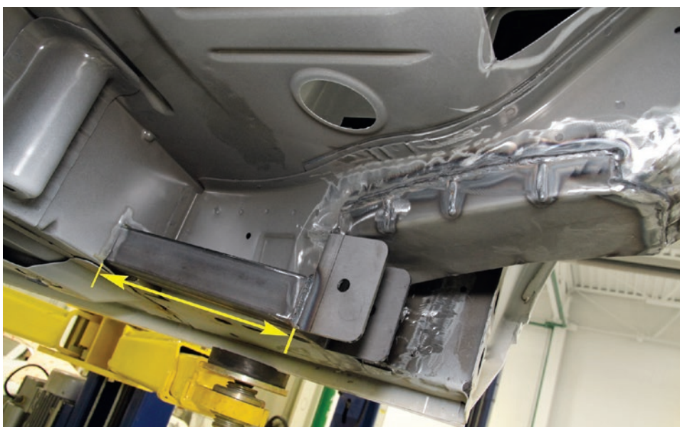
At their aft ends, the 2x2 subframe connector bars weld to the lower control-arm brackets. For reference, the dimension shown (unibody to rear face of LCA bracket) is 11.125 inches.
