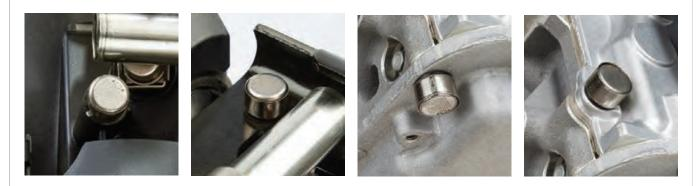
Engines are factory-sealed with tamper resistant seals to maintain engine integrity when used in NMCA drag racing class competition. Seals are engine specific and are designed for single-time use.
