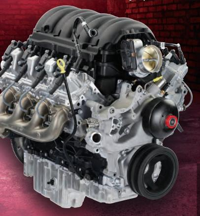
By combining the large–displacement and heavy–duty elements of the L8T 6.6L engine of the Silverado HD, a unique non–AFM (Active Fuel Management) LT2-based camshaft from of the Corvette Stingray's high-revving LT2 V-8, Chevrolet Performance engineers have created the all-new L8P performance crate engine - PN 19435523.
