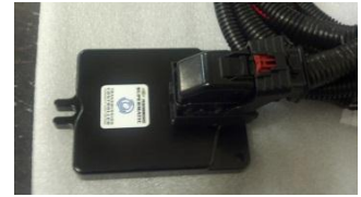
Transmission Control Unit Connection
