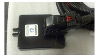
Transmission Control Unit Connection
