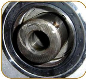
In Fig 15 you can clearly see the pin. It is located at the 2 o'clock position in the picture.
