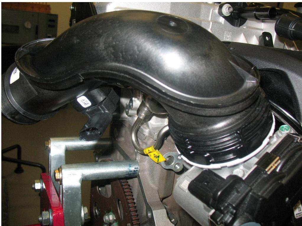
6. Tighten the clamp to 4 NM (35 lb in) once customer supplied tube/hose is in place. This tube is from the customer provided Charge air Cooler.
