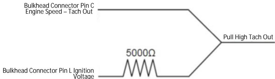
NOTE: When connected to the CHEVROLET PERFORMANCE Supermatic Connect and Cruise Harness the pull up resister is not required for the Transmission Controller.
