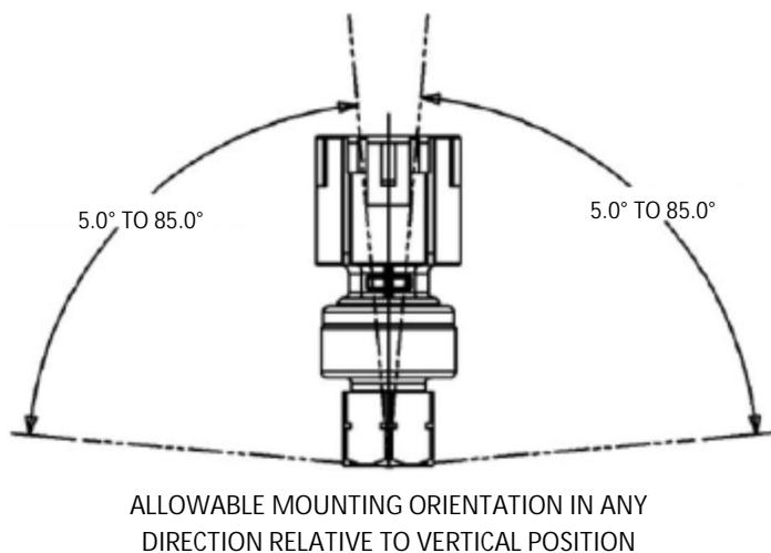
ALLOWABLE MOUNTING ORIENTATION IN ANY DIRECTION RELATIVE TO VERTICAL POSITION
