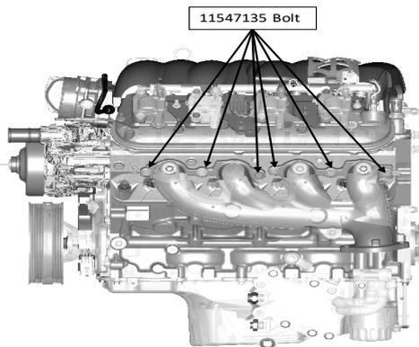
Install the exhaust manifold assemblies as shown below and torque the attachment bolts - 11547135 6 places per side - as follows:
