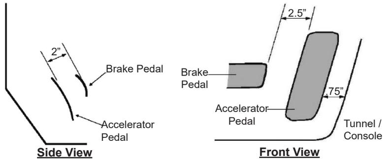
Mount the accelerator pedal per the following dimensional guidelines, mounting details are application-specific and are left to the user. Ensure that the pedal is securely mounted to the vehicle. A grommet is required in any sheet metal hole that the harness routes through to avoid wire damage.
