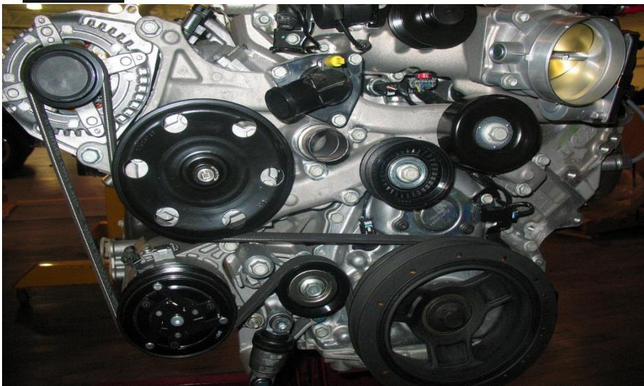
8. Install Super Charger Idler (12678295) and SC pulley (12642706) as shown in Figure 9 – torque to 58 NM (43 FT LB):
