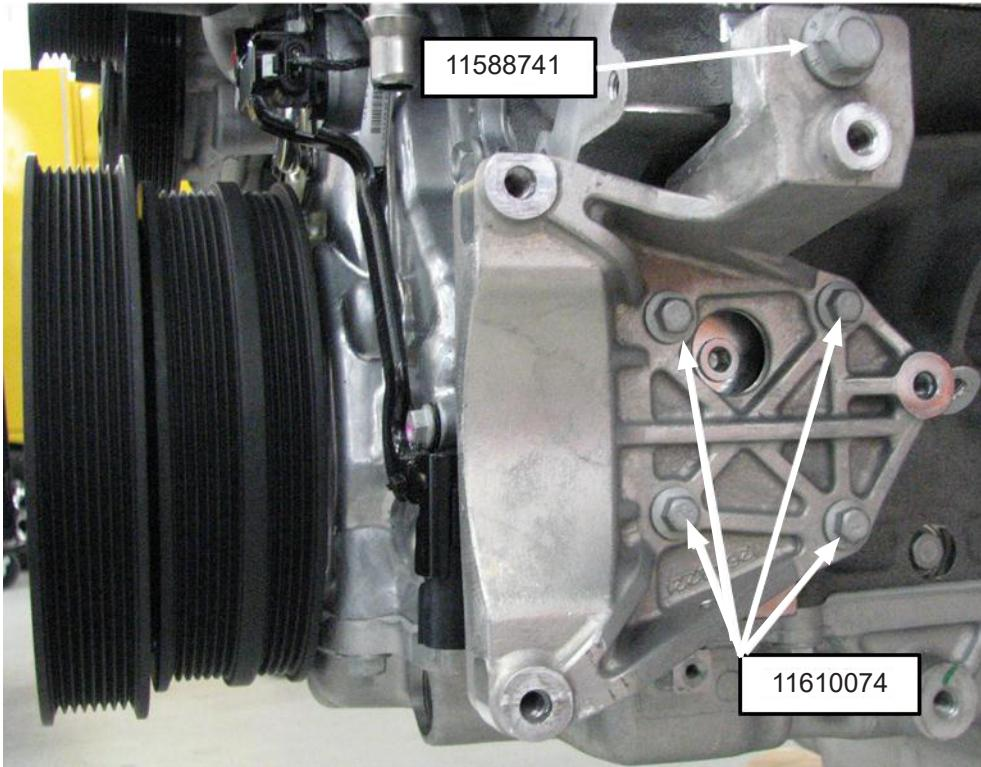
2. Install stud, 11561137 as shown in Figure 3. Torque to 8 N-M (71 LB-IN). Attach the Air Conditioning (A/C) compressor 23323121 to the bracket engine with bolts 11588732 and 11588735 as shown in Figure 3 and 4. Torque nut 11514596 to 22 N-M (16 LB-FT). Torque bolts 11588732 and 11588735 to 25 N-M (18 LB-FT).
