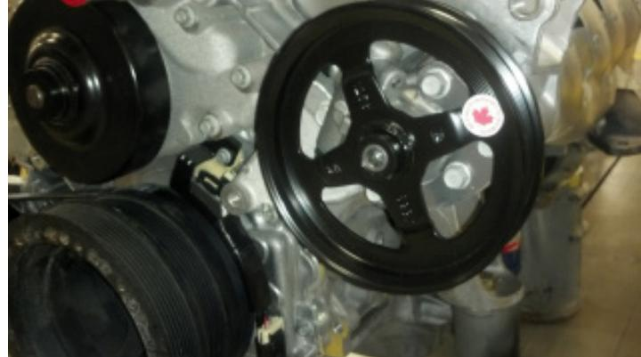
5. Install 25888970 Generator onto bracket using bolts 24503609 (2).
