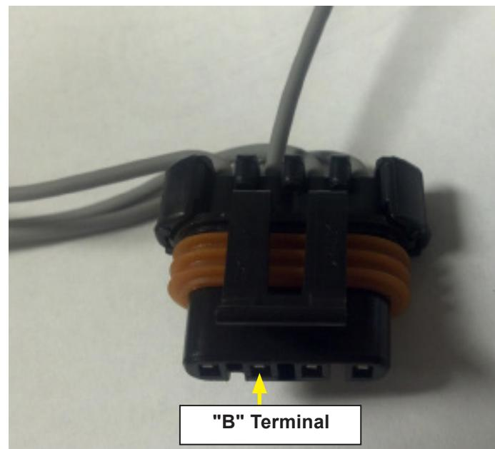
Remove original Generator connector from Chevrolet Performance Parts LSA engine harness and splice wire from cavity "B" on 15306009 connector into orange wire from LSA engine harness. Other wires in connector are unused.
