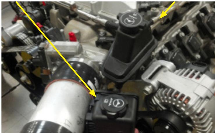
Inner fender mount may also be used. Must be positioned higher than the pump. Hose from reservoir to pump is not included in this kit. Must obtain locally.
