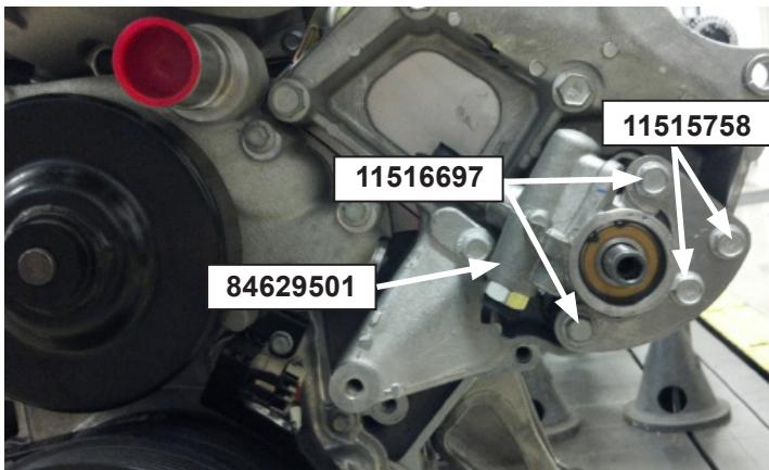
4. Install P/STG pump pulley 12568997 onto pump using a power steering pump pulley installation tool (not included). The part number on the pulley faces away from the pump. Install the pulley until the outer edge of the hub is flush with the end of the pump shaft. See figures 3 and 4 below.
