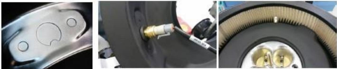
In the Air Cleaner base, that is a component included in the ZZ6 Air Cleaner Kit supplied with the ZZ6 "Turn Key" package, (1) remove the formed round knockout panel, (2) insert the supplied rubber grommet and (3) install the MAT Sensor in the grommet. Connect the wire lead, labelled "Air Temp", from the wiring harness to the MAT Sensor as shown above.
