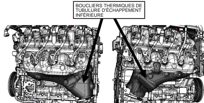
BOUCLIERS THERMIQUES DE TUBULURE D'ÉCHAPPEMENT INFÉRIEURE
