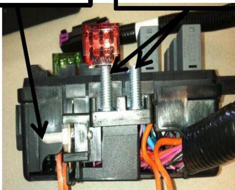
Attach a 12 volt ignition switch feed from the vehicle to the pink ignition switch wire in the harness (this is required to enable the proper power-up sequence of the ECM). This can be routed into the passenger compartment with the accelerator pedal connector and diagnostic link connector. Next, connect battery power (minimum 8 gauge wire) to the horizontal stud on the fuse relay center. The other two studs are for accessories and are 50 amp fused), and the harness installation is complete.
