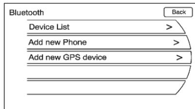
3. Turn the MENU/SEL knob until Device List displays. Press the MENU/SEL knob or press the Device List screen button to display other options.
