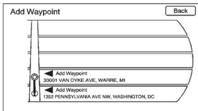
Up to three waypoints can be added to the current route, between the start point and final destination. The waypoints can be edited or deleted.
