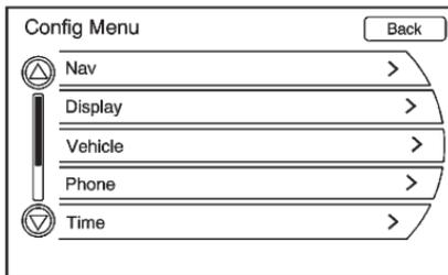
1. Press the CONFIG button. Turn the MENU/SEL knob until the Phone menu displays. Press the MENU/SEL knob or press the Phone screen button to display other options.
