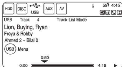
A USB Mass Storage device can be connected to the USB port to copy compressed audio files onto the hard drive. Content can also be played directly from the USB device.
