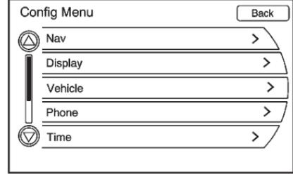
To scroll through the available setup options, press the CONFIG button to display the Config Menu features. Turn and press the MENU/SEL knob or press the desired option.
