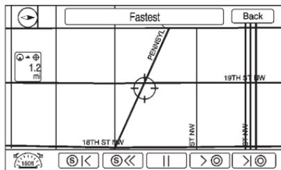
**< > (Reverse or Forward Skip) :** Press the reverse skip arrow to go to the start point. Press the forward skip arrow to go to the final destination.
