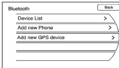
3. Select "Add New Phone." Start the pairing process on the cell phone that you want to pair. See the cell phone manufacturer's user guide for information on this process.
