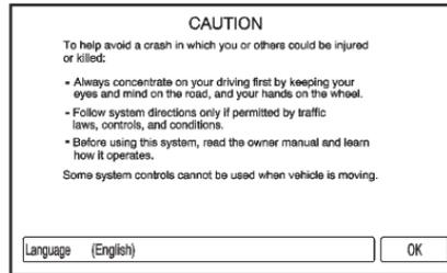
Each time the vehicle is started and the navigation system is turned on, the Caution screen appears. Press OK to accept the Caution. If OK is not selected, all buttons except for NAV (Navigation) and DEST (Destination) can be accessed.
