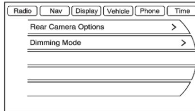
Press the CONFIG button to enter the Setup menu features. Turn the MENU/SEL knob until Display appears, then press the knob or press the Display screen button.
