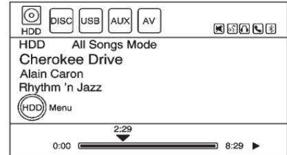
Press the HDD/DVD/AUX button; cycle through the available audio source until the HDD source displays or press HDD/DVD/AUX once, and press the HDD source button.
