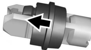
8. Verify the retainer ring is in the proper position. If the retainer ring is out of position, it will not engage. Reset the retainer by pulling it forward with a tool.
