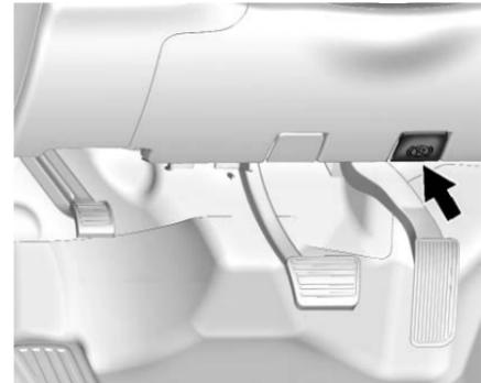
For vehicles with a release handle, set the parking brake by holding the regular brake pedal down, then pushing down the parking brake pedal.
