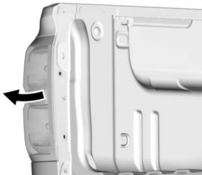
4. Pull the rear lamp assembly straight back to remove it from the vehicle.
