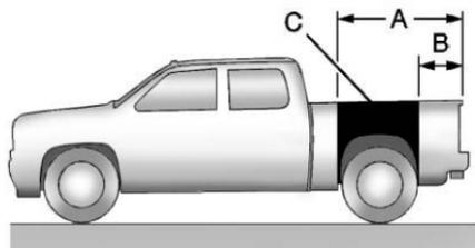
Use the rear edge of the load floor for measurement purposes. The recommended location for the cargo center of gravity is at point C for the CWR. It is the point where the mass of a body is concentrated and, if suspended at that point, would balance the front and rear.
