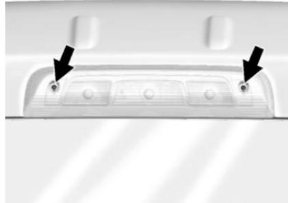
1. Remove the two screws and lift off the lamp assembly.
