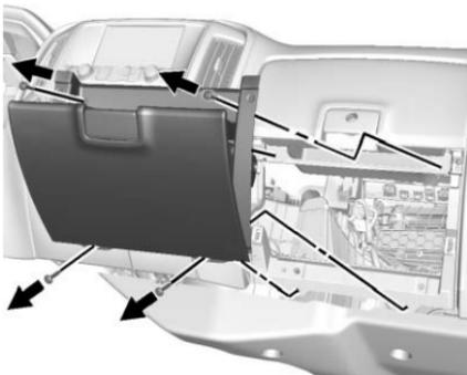
3. Close the lower glove box door and pull it from its frame to remove the entire unit.
