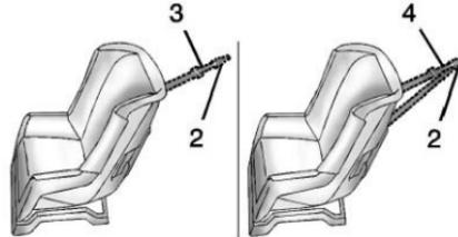
A top tether (3, 4) anchors the top of the child restraint to the vehicle. A top tether anchor is built into the vehicle. The top tether attachment (2) on the child restraint connects to the top tether anchor in the vehicle in order to reduce the
