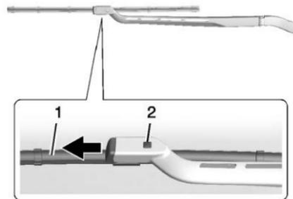
2. Press the button (2) in the middle of the wiper arm connector, and pull the wiper blade away from the arm connector (1).
