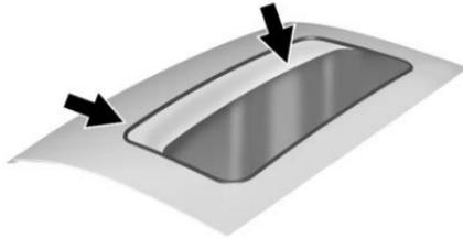
Dirt and debris may collect on the sunroof seal or in the track. This could cause an issue with sunroof operation or noise. It could also plug the water drainage system. Periodically open the sunroof and remove any obstacles or loose debris. Wipe the sunroof seal and roof sealing area using a clean
