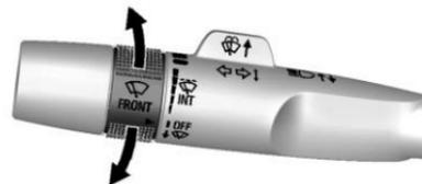
The windshield wiper control is on the turn signal lever.
