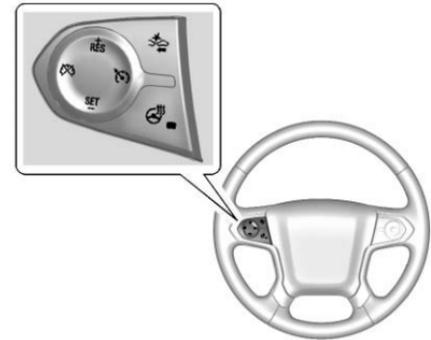
The Collision Alert control is on the steering wheel. Press
