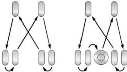
Use this rotation pattern when rotating the tires if the vehicle has dual rear wheels (except polished forged aluminum wheels).
