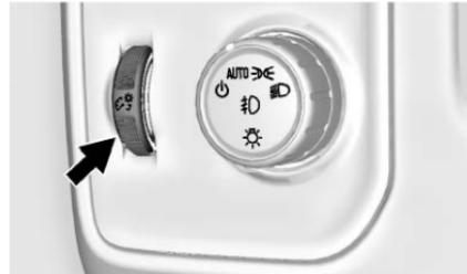
This feature controls the brightness of the steering wheel and instrument panel lights. The instrument panel illumination control is next to the exterior lamp control.
