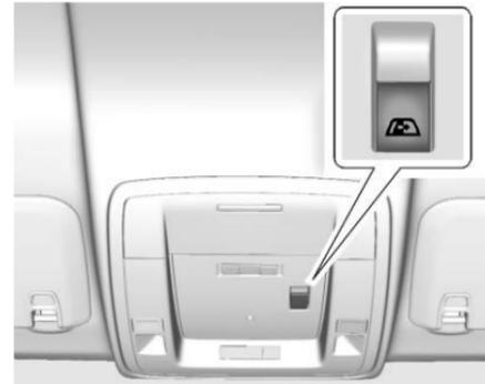
If equipped, the power sliding rear window works when the ignition has been turned to ACC/ACCESSORY or ON/RUN, or when Retained Accessory Power (RAP) is active. See *Retained Accessory Power (RAP)* ⇨ 271.
