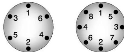
13. Tighten the nuts firmly in a crisscross sequence, as shown, by turning the wheel wrench clockwise.
