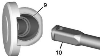
3. Insert the hoist end (open end) (10) of the extension through the hole (9) in the rear bumper.
