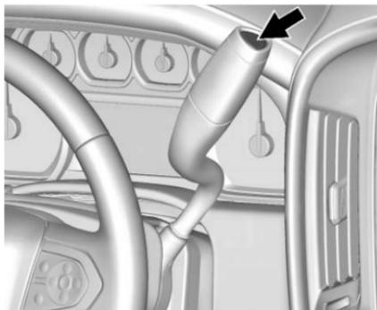
Vehicles with an automatic transmission have a Tow/Haul Mode. The Tow/Haul Mode adjusts the transmission shift pattern to reduce shift cycling. This provides increased performance, vehicle control, and enhanced transmission and engine cooling when driving down steep hills or mountain grades, when towing, or when hauling heavy loads.
