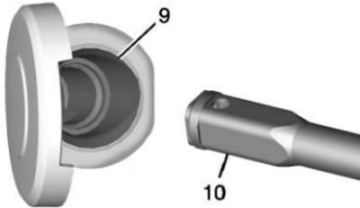
4. Insert the hoist end (10) through the hole (9) in the rear bumper and onto the hoist shaft.
