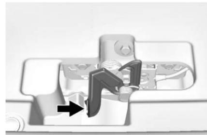
2. Go to the front of the vehicle to find the secondary hood release. The handle is under the front edge of the hood near the center. Push the handle to the right and at the same time raise the hood.
