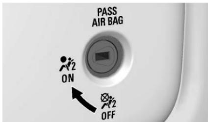
To turn the front outboard passenger frontal airbag on again, insert the ignition key into the switch, push in, and move the switch to the on position.
