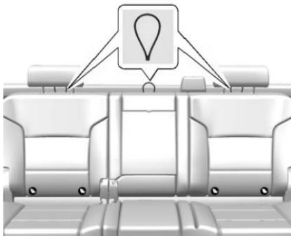
The top tether anchors are the loops near the top of the seatback for each rear seating position. These loops will be used to route the top tether through, as well as to secure the top tether to the vehicle. Be sure to use the anchor (loop) on the same side of the vehicle as the seating position where the child restraint will be placed.
