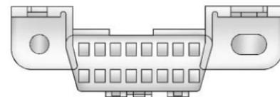
The DLC is under the instrument panel to the left of the steering wheel. Connecting devices that are
