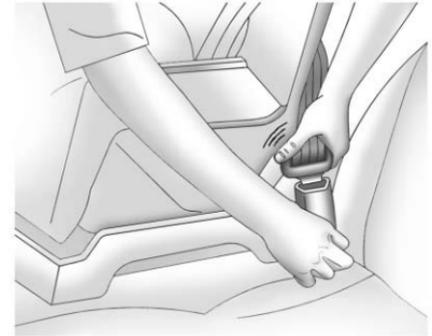
4. Push the latch plate into the buckle until it clicks. Position the release button, away from the child restraint system, so that the safety belt could be quickly unbuckled if necessary.
