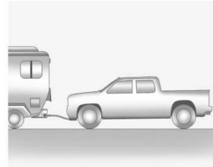
Only dinghy tow four-wheel-drive vehicles with a two-speed transfer case that have an N (Neutral) and a Four-Wheel Drive Low (4 ↓) setting.
