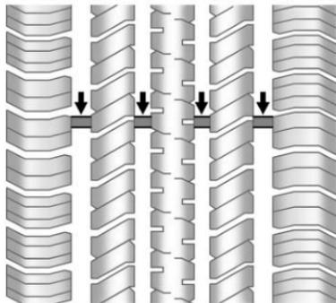
Treadwear indicators are one way to tell when it is time for new tires. Treadwear indicators appear when the tires have only 1.6 mm (1/16 in) or less of tread remaining. Some commercial truck tires may not have treadwear indicators. See *Tire Inspection* ⇨ 411 and *Tire Rotation* ⇨ 412 for additional information.
