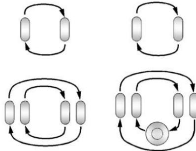
Use this rotation pattern when rotating the tires if the vehicle has polished forged aluminum dual rear wheels. The spare wheel can be used in any position in the event of a flat tire, and can be rotated with the rear
