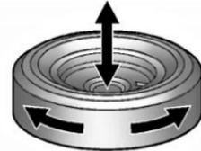
7. Make sure the tire is stored securely. Push, pull, and then try to turn the tire. If the tire moves, use the wheel wrench to tighten the cable.
