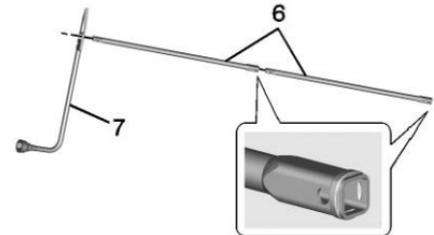
2. Assemble the wheel wrench (7) and the two jack handle extensions (6), as shown.
