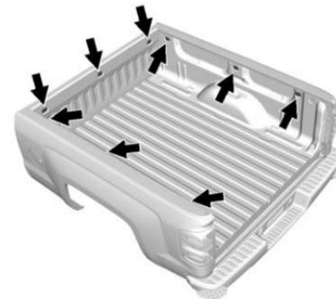
The vehicle may be equipped with cargo tie-downs.
