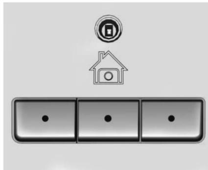
If equipped with the Universal Remote system, these buttons will be in the front overhead console.
