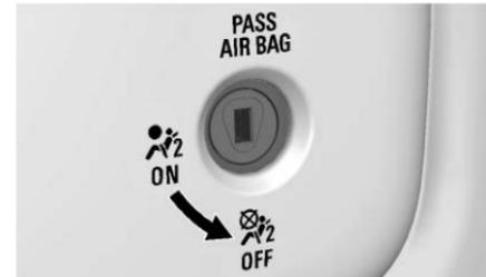
To turn off the front outboard passenger frontal airbag, insert the ignition key into the switch, push in, and move the switch to the off position.
