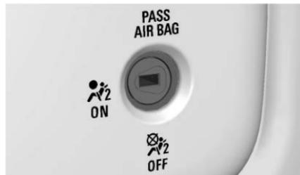
If the vehicle does not have an airbag on-off switch, it may have a passenger sensing system. See *Passenger Sensing System* ⇨ 82.
