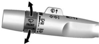
The windshield wiper control is on the turn signal lever.
