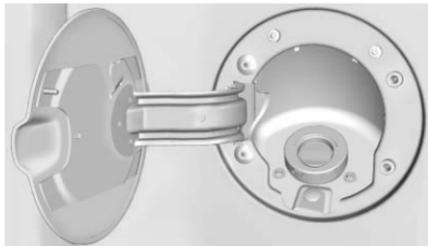
The vehicle has a capless refueling system and does not have a fuel cap. The filling nozzle must be fully inserted and latched prior to starting fuel flow.
