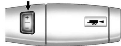
The Range Selection Mode buttons, if equipped, are on the automatic transmission shift lever.
