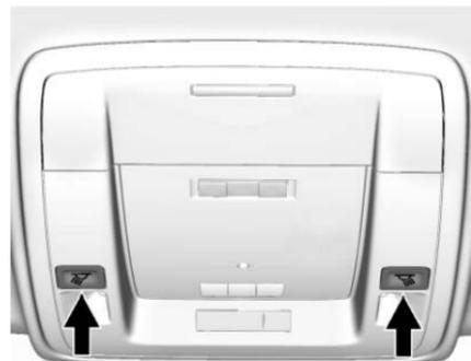
There are reading lamps in the overhead console and the headliner, if equipped. To operate, the ignition must be in the ACC/ACCESSORY or ON/RUN position or using Retained Accessory Power (RAP).
