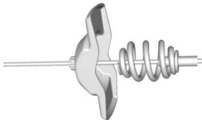
Tilt the retainer and pull it through the center of the wheel along with the cable and spring.
