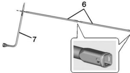
3. Attach the wheel wrench (7) and extensions (6) together, as shown.
