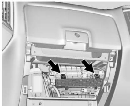
4. Release the two tabs holding the service door. Open the service door and remove the old filter.
