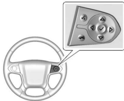
△ or ▽ : Press to move up or down in a list. In the main view, you can press up and down to move between different info app pages.
