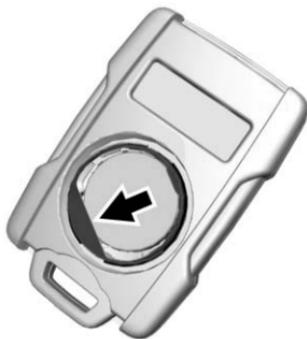
2. Press and slide the battery down toward the pocket of the transmitter in the direction of the key ring. Do not use a metal object.
