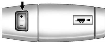
If equipped, Range Selection Mode helps control the vehicle's transmission and vehicle speed while driving downhill or towing a trailer by letting you select a desired range of gears.
