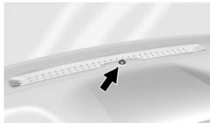
There is a light sensor on top of the instrument panel. Do not cover the sensor, otherwise the headlamps will come on when they are not needed.
