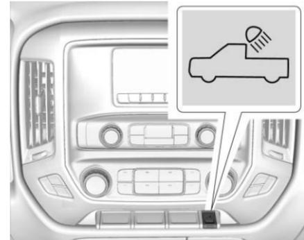
The cargo lamp provides more light in the cargo area or on the sides of the vehicle, if needed. The lights inside the pickup box and/or on the outside rearview mirrors also turn on, if equipped.
