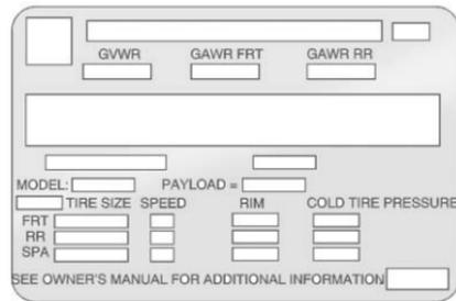
A vehicle-specific Certification/Tire label is label is attached to the center pillar (B-pillar). The label may show the size of the vehicle's original tires and the inflation pressures needed to obtain the gross weight capacity of the vehicle. This is called Gross Vehicle Weight Rating (GVWR). The GVWR
