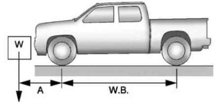
$(W \times (A + W.B.)) / W.B. =$  Weight the accessory is adding to the front axle.
