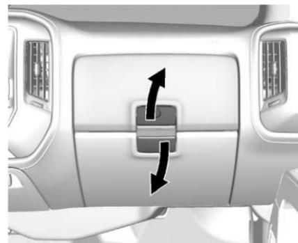
To access the upper glove box, unlock with the key and pull up on the handle.
