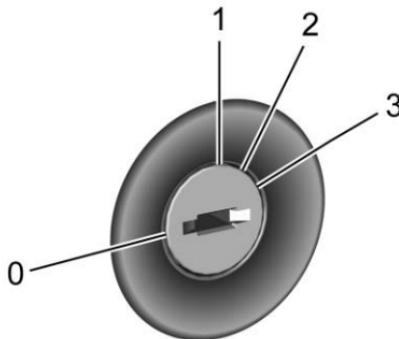
The ignition switch has four different positions.
