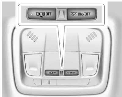
Dome Lamp Controls
