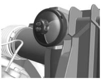
If the gauge is in the red zone, replace the air cleaner/filter and then reset the gauge by twisting the black knob until the gauge is in the complete green zone.
