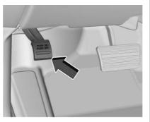
Set the parking brake by holding the regular brake pedal down, then pushing down the parking brake pedal. If the ignition is on, the brake system warning light will come on. See Brake System Warning Light ⇔ 115.
