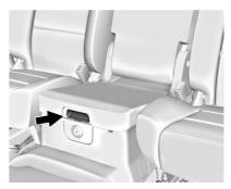
If equipped with front seat floor console storage, unlock with the ignition key, press the button, and lift to open.
