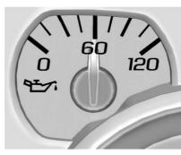
The engine oil pressure gauge shows the engine oil pressure in psi (pounds per square inch) when the engine is running.
