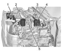
Radiator and Charge Air Cooler: Check for loose mounting and damage. Inspect condition of all hoses for damage, cracks, and leaks. Inspect for foreign material on face of cooling package. Carefully brush away collected materials without bending cooling fins to maintain proper airflow through cooling package.
