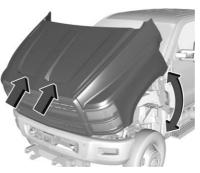
Carefully tilt the hood forward using the front of the hood, where indicated by arrows, until it comes to a vertical stop.
