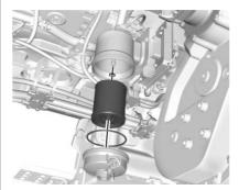
3. Remove the filter element cap by turning it counterclockwise.
