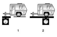
The trailer tongue weight (1) should be 10–15% and fifth-wheel or gooseneck kingpin weight should be 15–25% of the total loaded trailer weight (2). Some specific trailer types, such as boat trailers, fall outside of this range. Always refer to the trailer owner's manual for the recommended trailer tongue weight for each trailer. Never exceed the maximum loads for your vehicle, hitch and trailer.
