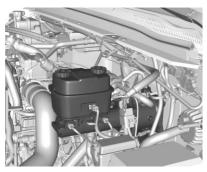
Check and refill the brake fluid reservoir:
