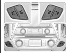
If equipped, the buttons are on the center stack. To operate, the engine must be running.
