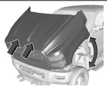
Carefully tilt the hood back using the front of the hood, where indicated by arrows, until it is lowered all the way.
