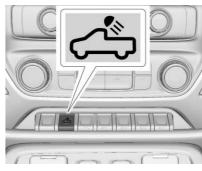
The cargo lamp provides more light in the cargo area or on the sides of the vehicle, if needed. The lights on the outside mirrors also turn on, if equipped.
