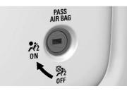
To turn the front outboard passenger airbag on again, insert the ignition key into the airbag on-off switch, push in, and move the switch to the ON position.
