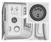
Use the transfer case knob, next to the steering wheel, to shift into and out of four-wheel drive for extra traction. All of the lights will flash on then off momentarily when the ignition is turned on. The light that remains on will indicate the state of the transfer case.
