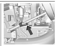
3. The hood actuator lock, located on the passenger side, will lock to secure the hood.
