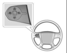
S: Press to turn the system on or off. The indicator light is white when cruise control is on and turns off when cruise control is off. **+RES** : If there is a set speed in memory, press briefly to resume to that speed or press and hold to accelerate. If cruise control is already active, use to increase vehicle speed.
