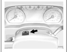
A: Press this button to make the front and rear turn signal lamps flash on and off. Press again to turn the flashers off.
