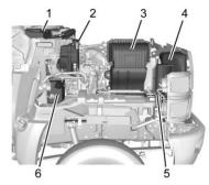
1. Cowl Vent: Ensure the air inlet cover is free of dirt and debris.
