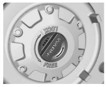
The locking hubs are located on each end of the front axle and must be manually turned to LOCK before the four-wheel drive modes can be used.
