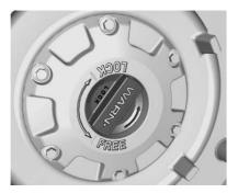
The locking hubs are on each end of the front axle and must be manually turned to LOCK before the four-wheel drive modes can be used.
