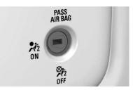
To operate the airbag on-off switch, use the vehicle key.
