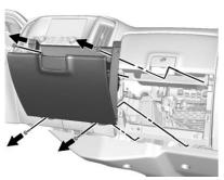
Close the lower glove box door and pull it from its frame to remove the entire unit.
