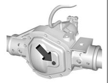
The fluid level should be even with the bottom of the fill plug hole. Add only enough fluid to reach the proper level.
