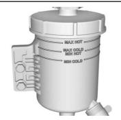
2. Check to see if the fluid level is at or above the MIN HOT level and below the MAX HOT level if the fluid is hot, or if the fluid level is at or above the MIN COLD level and below the MAX COLD line if the fluid is cold.
