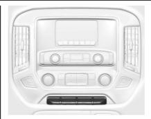
To activate the system, press the exhaust brake switch. A light in the switch will come on when the exhaust brake is activated. The switch must be pressed at each vehicle start for the system to be active.
