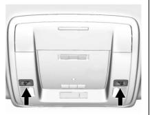
There are reading lamps in the overhead console and the headliner, if equipped. To operate, the ignition must be on or in ACC/ACCESSORY or using Retained Accessory Power (RAP).
