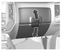
To access the upper glove box, unlock with the key and pull up on the handle. There may be a USB port in the upper glove box. See  $USB Port \Rightarrow 160$ .
