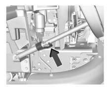
Lift up on the hood actuator strut lock, located on the passenger side, to unlock the actuator strut and allow the hood to be closed.
