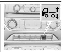
The system is controlled by the Air Suspension Dump (ASD) switch in the center stack. This switch controls solenoids, which direct air to the suspension dump and height valve.
