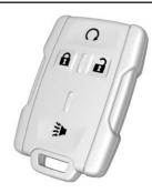
**1** : Press to unlock the driver door. Press **1** again within three seconds to unlock all remaining doors.
