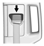
Push down on the release button to move the height adjuster to the desired position.
