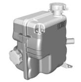
The coolant surge tank is divided into two sides. The upper portion coolant level should be at or above, the bottom of the indicator arrows. The coolant level must be checked when the engine is cold and the vehicle must be on a level surface.
