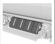
The batteries are located on the outboard side of the left frame rail, under the cab. The batteries are in a carrier with the cover retained by hold down straps.
