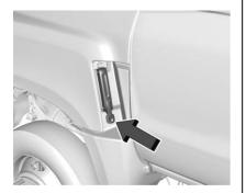
Go to the driver side of the vehicle and pull up on the hood latch, then go to the passenger side and pull up on the other hood latch.
