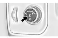
If equipped, the control is on the center of the exterior lamp control, to the left of the steering column.
