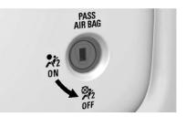
To turn off the front outboard passenger frontal airbag, insert the ignition key into the airbag on-off switch, push in, and move the switch to the OFF position.
