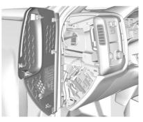
The left instrument panel fuse block access door is on the driver side edge of the instrument panel.
