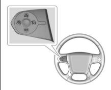
S: Press to turn the system on or off. The indicator light is white when cruise control is on and turns off when cruise control is off.
