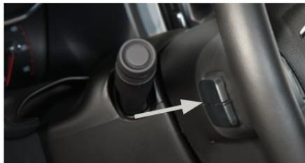
If equipped with the color Driver Information Center, the Next/Previous Favorite Station buttons (shown) and the Volume buttons are located behind the steering wheel.
