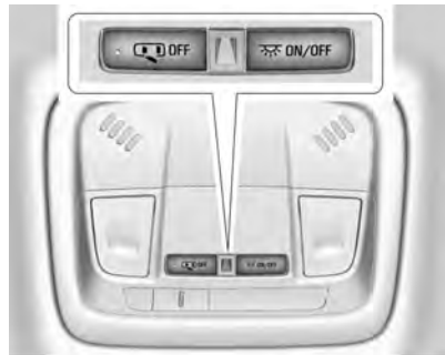
Dome Lamp Controls
